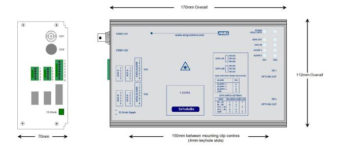
The **AMG5714A1B9-HP** is a standalone one channel video receive unit designed to receive 1 video signal and transmit & receive 2 data signals, 1 Bi-directional alarm, plus 1 Bi-directional audio channel over a single Singlemode optical fibre.
